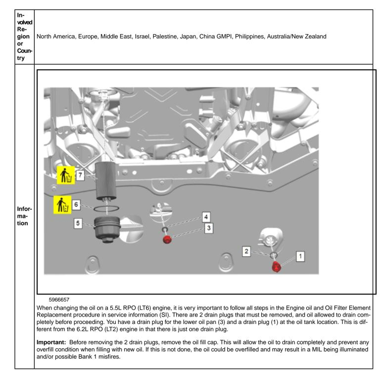
There have been cases where one of the drain plugs has not been removed and upon adding new engine oil, the engine can now become overfilled with oil, leading to potential driveability and/or engine damage concerns.
