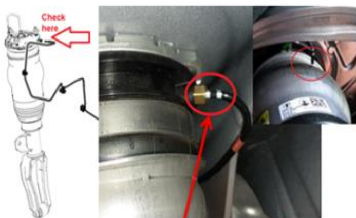
Sample of incorrect Air Suspension pipe installation on the front Air spring
