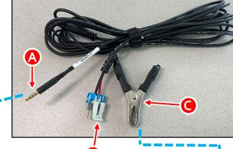
3. Disconnect the knock sensor connector and connect the knocking sensing connector of the engine vibration inspection harness to the engine knock sensor (B).
