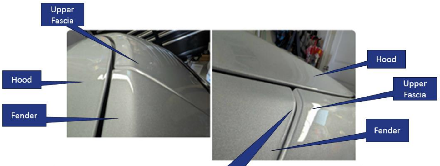
Fender to Fascia Gap/Flush Issues
