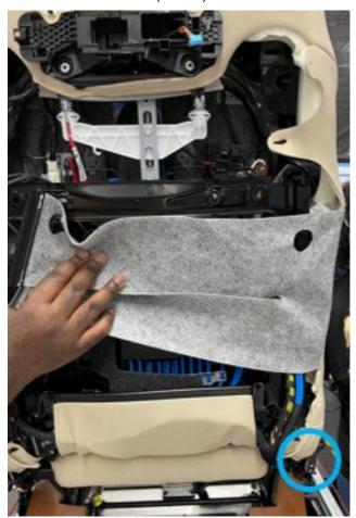
The eyelet on the ground wire should make solid connection to the structure with no free play.
