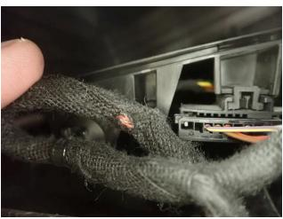
This shows the harness damage; the sheathing has been abraded.
