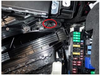
This is where the harness can be damaged when installing the cabin air filter cover screw.
