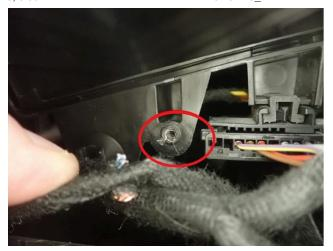
With the harness pulled out of the way, you can see the screw mounting hole for the cabin air filter cover
