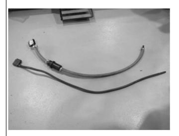
A filter may be installed between the EVAP canister and air inlet, to correct this Condition. An example of the original, and the retro-fit, evaporative emission canister vent hose are shown in the graphic above.
