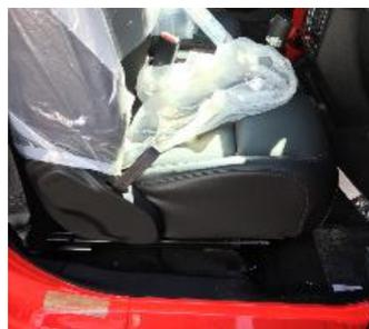
Step 3. Remove the 4 bolts that hold the seat to the truck floor and discard. The bolts have lock patch that is not reusable.
