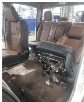
Step 5. Remove the fore/aft wire harness motor connector from the fore/aft motor (back right of the seat adjuster). Push on the tab to remove the motor wire harness connector from the motor. Leave disconnected for 10 seconds.
