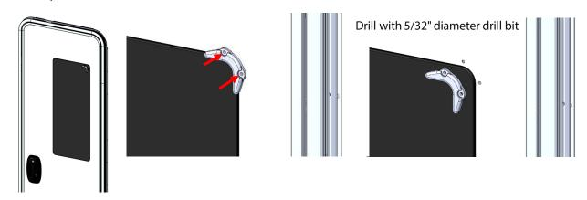
Increase the diameter from 5/32" to 5/16", drilling with 5/16" (8mm) drill bit.
