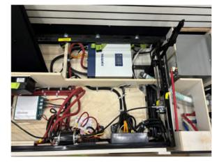
Disconnect the 120v wiring, 12v wiring, RV-C connection and BTS (battery temperature sensor).
