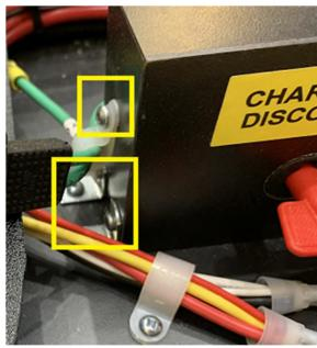
THEN WITH THE BOX PULLED FORWARD, ACCESS THE REAR OF THE DISCONNECT BOX AND REMOVE THE WIRES CONNECTED TO THE INPUT AND OUTPUT POSTS OF THE KEY. KEEP IN MIND WHICH WIRES WENT TO WHICH POSTS FOR WHEN YOU REINSTALL THEM ONTO THE NEW KEY.
