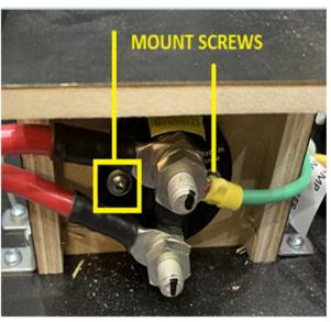
LASTLY, REMOVE THE 2 SCREWS THAT SECURE THE CHARGE LINE DISCONNECT KEY TO THE BACK OF THE BOX. THEN SLIDE IN THE NEW DISCONNECT KEY IN PLACE AND SECURE, HOOK WIRES BACK TO ORIGINAL POSTS AND REMOUNT THE CHARGE LINE DISCONNECT BOX ONTO THE TOP OF THE BATTERY BOX.
