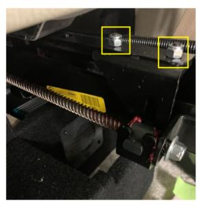
Insert a screw driver into the frame at this location and move the mechanism side to side to free up any binding that may be occurring. The sofa may also shift slightly once these bolts are loosened. The sofa should settle into a position that will not cause it to bind. Run the sofa down fully and then retract fully. Tighten down the 7/16" nyloc nuts to complete.
