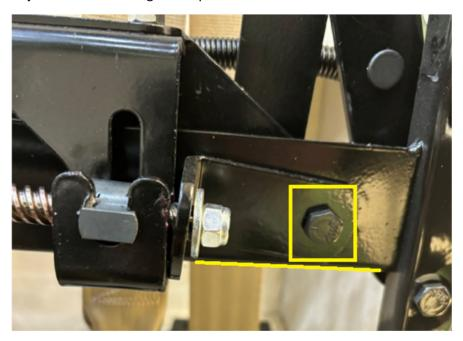
Then loosen the (4) 7/16" nyloc nuts on both passenger and driver side screw rod brackets.
