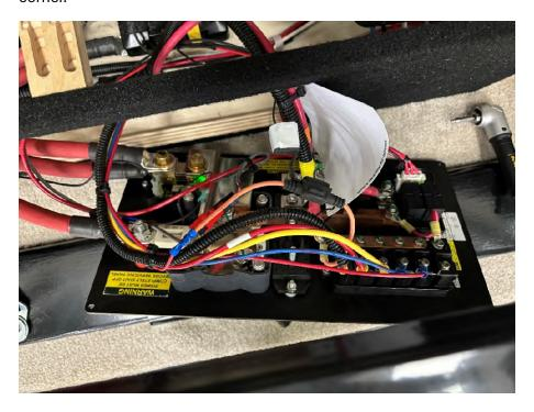
On the Trustate Monitor, disconnect the thermistor (white plug with 2 black wires):
