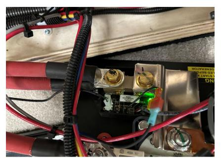
\*Tape these 2 red cables as carefully set aside making sure they do not touch anything grounded. These lines are live with 12v + from the batteries. The metal bar that secures the seatbelts at the back of the coach for example is grounded.
