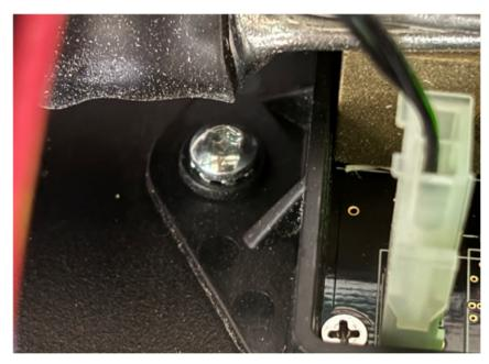
Slide the new module into position and secure the Torx screw first. Then work your way in reverse order to re-install the replacement module. The brass colored bolts are torqued to 100" lbs. Once completed, access the rear touch screen in the coach and follow the prompts for update master.
