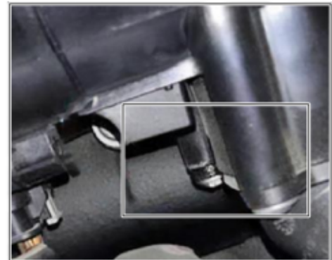
Slight traces of coolant (current type of coolant regulator with a leakage tank)
