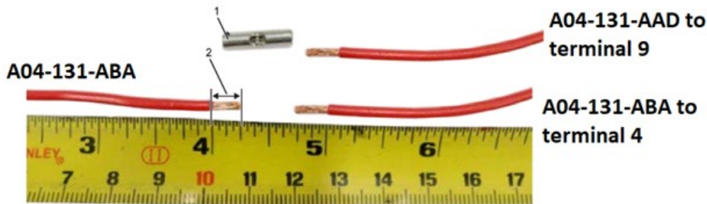
Figure: Insulation Stripped 1/4 inch
