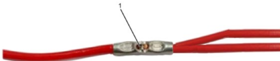
Figure: Crimp Splice Crimped on Both Wires
