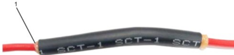
Figure: Dual Wall Heat Shrink Sleeve Over Splice
