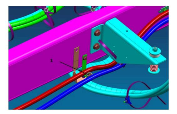
3. Replace the removed saddle bracket with pn: 3821016C1 shown on the right below; torque fastener to 41-50 lb-ft (56-68 Nm).
