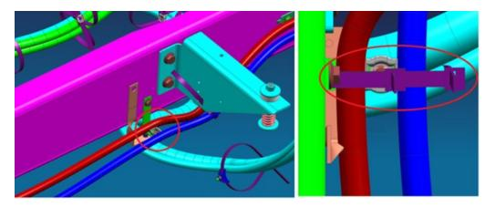
2. Remove the bolt (1) holding the saddle bracket to frame bracket (shown below). Keep the removed fastener, as it will be reused.
