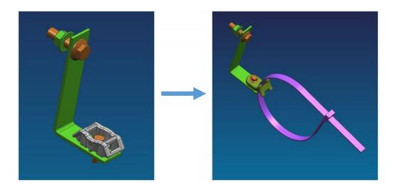
4. Using 3626607C1 Cable Lock, strap hoses to the saddle on the bracket shown below. Ensure the hoses do not touch the twisted AC bracket.
