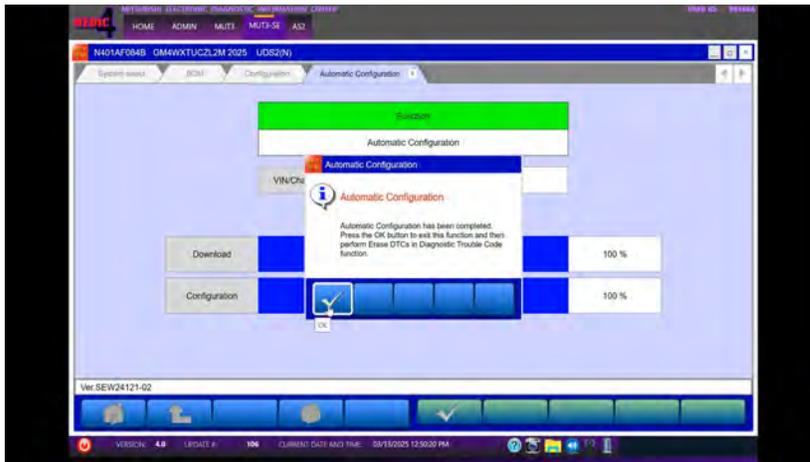
j. Press the "ALL DTCs" button and then press the "Erase and Read all DTCs" button. Press the "OK" button to begin. When completed press the "OK" button.
