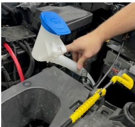
Figure 6. Set aside washer solvent filler neck.
