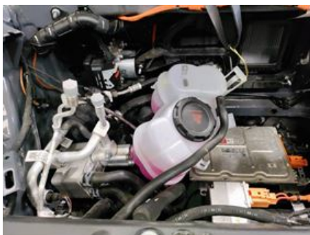
Figure 4. Coolant reservoir set aside.
