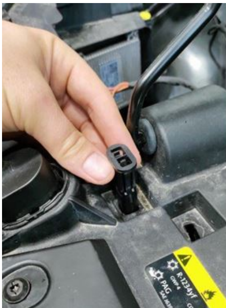
Figure 6. Set aside washer solvent filler neck.
