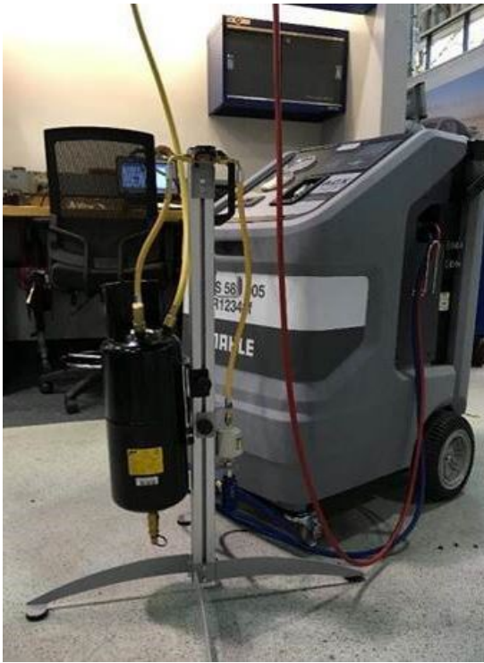
Figure 1. VAS581005 Air Conditioning Service System with Flushing Device.
