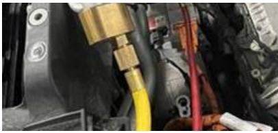
Figure 18. Installation of VAS 6338/3 and 6338/12.
