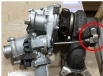
Illustration 1) wastegate rod (affected area on turbocharger)
