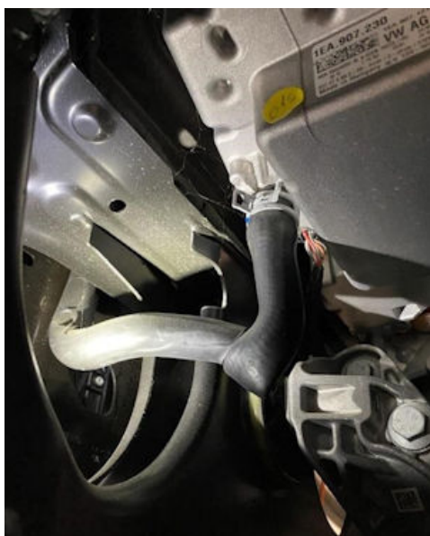
Figure 1. Hose twisted at rear power electronics.
