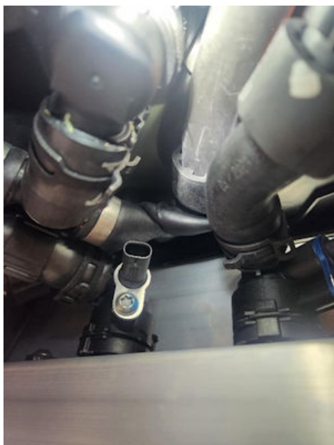
Figure 3. Hose twisted at front of high-voltage battery.
