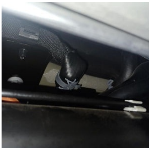
Figure 2. Hose twisted at rear power electronics.
