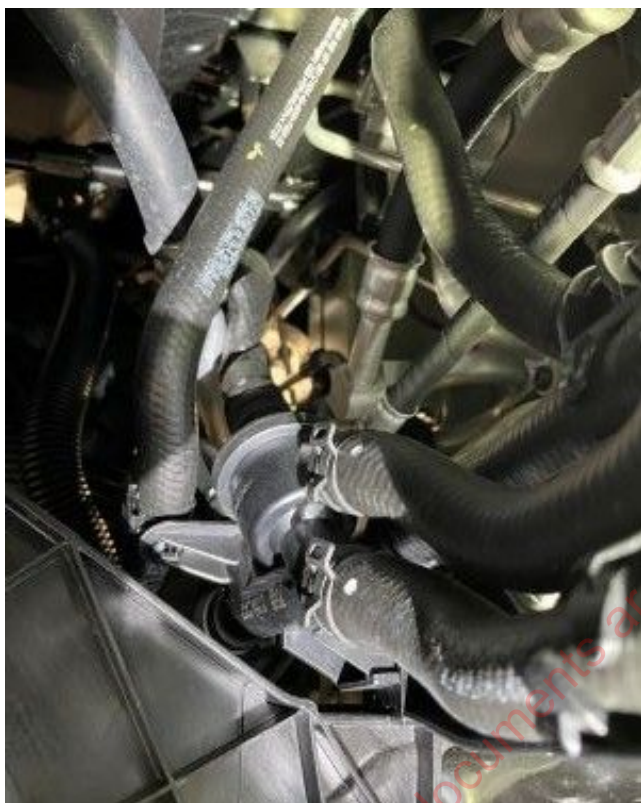
Figure 5. Hose twisted at thermostat.
