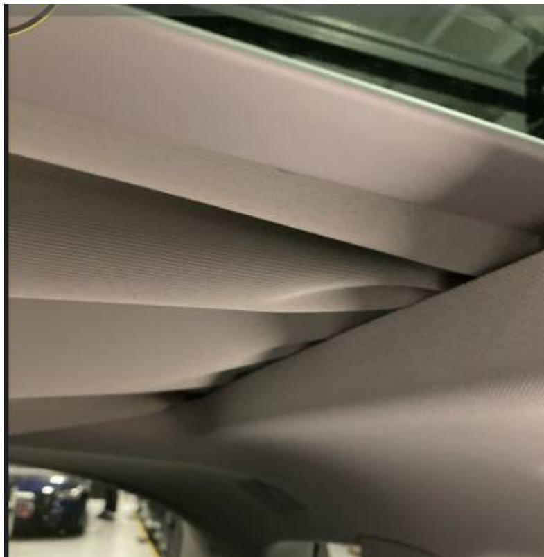
Figure 1. Material does not fold. Slider on left or right is stuck.
