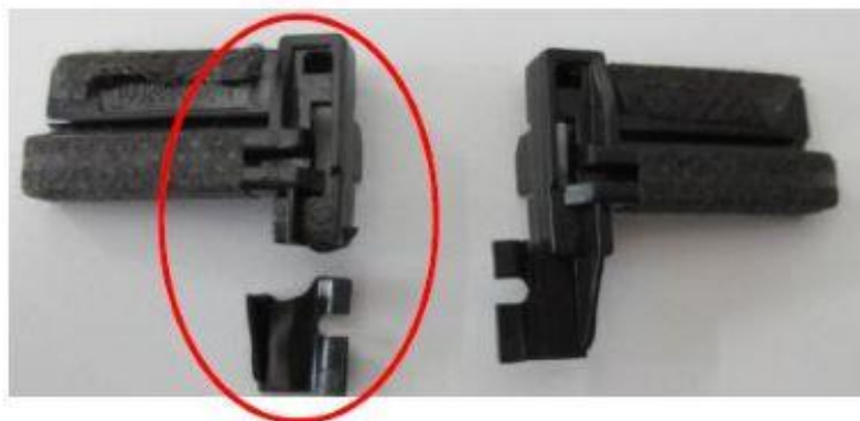
Figure 2. Broken slider left / unbroken slider right.
