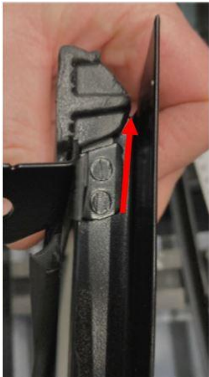
Figure 2. Gap between foam piece and the guide.
