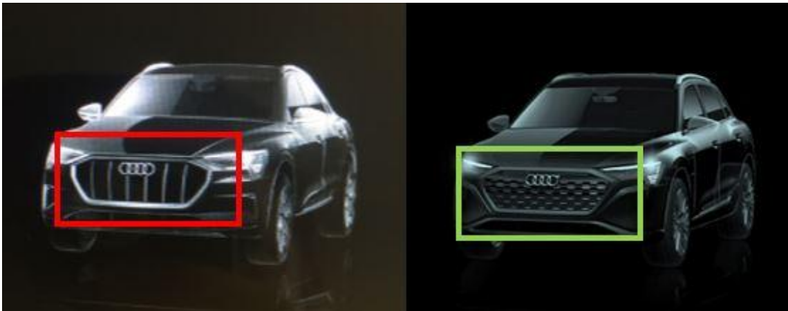
Figure 1. Radiator grille with lines (left, red rectangle) and honeycomb grille (right, green rectangle).
