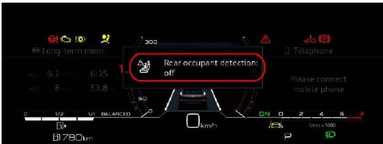
Figure 3. Rear occupant detection off message.
