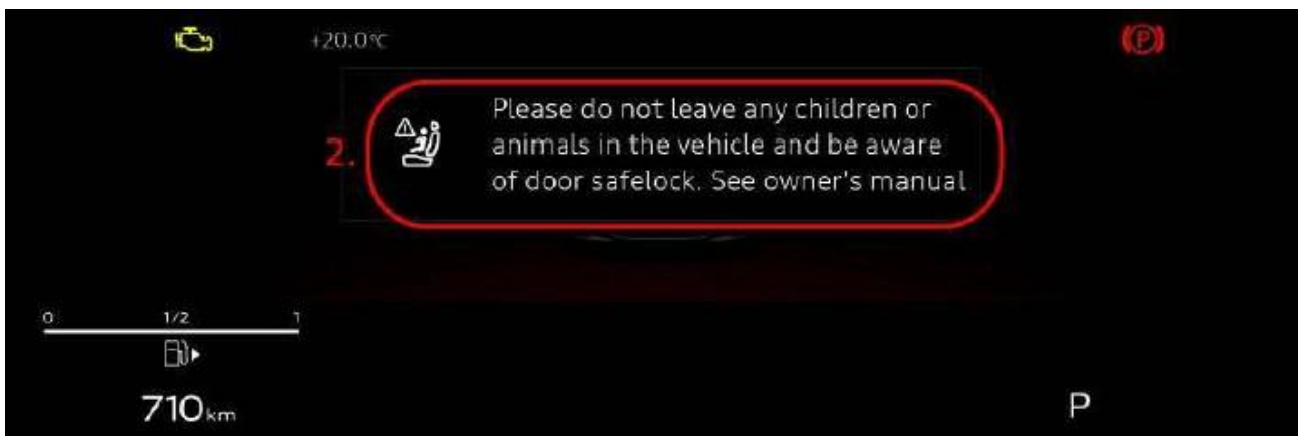
Figure 5. Rear occupant detection is switched off.
