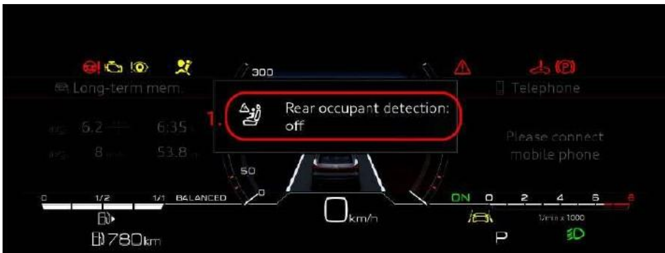
Figure 5. Rear occupant detection is switched off.
