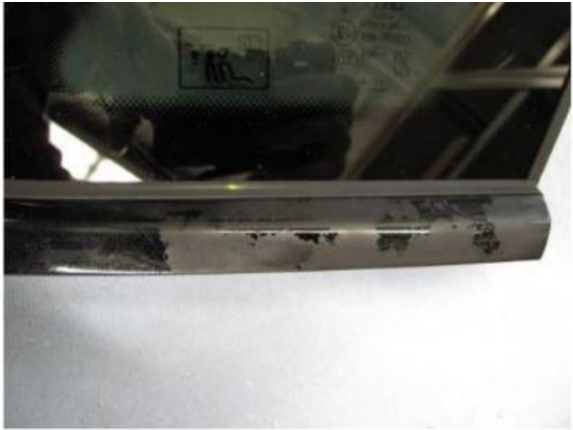
Figure 2. Coat peeled off.
