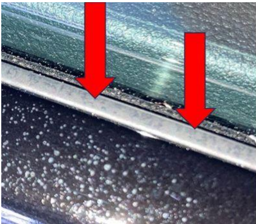
Figure 5. Marks forming caused by applied liquid.
