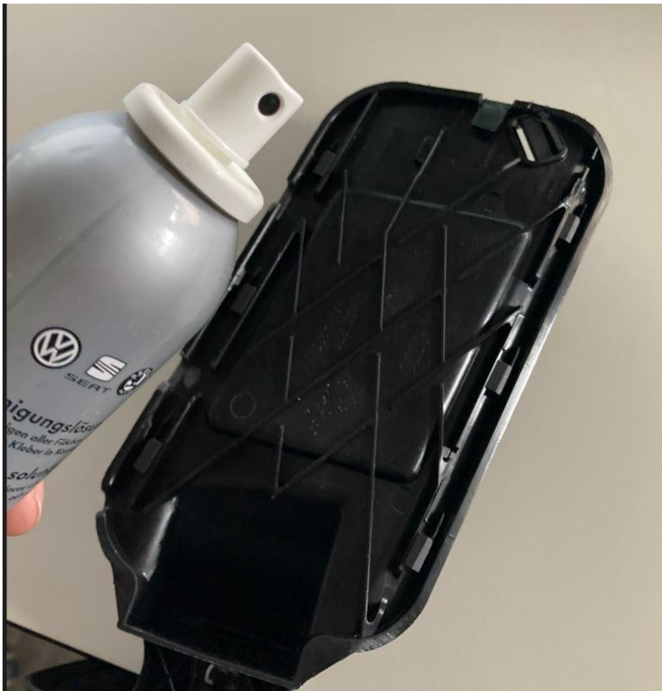
Figure 5. Clean the area which makes contact with the tank flap as well as the painted reverse side of the tank flap.
