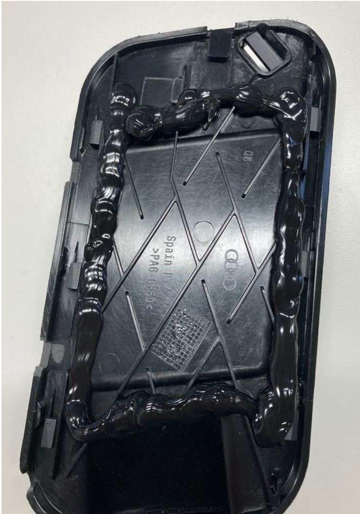
Figure 6. Adhesive applied to the bracket.
