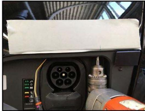
Figure 12: Use an angled drill/angle bit to drill to a depth of 15mm at the marked location.
