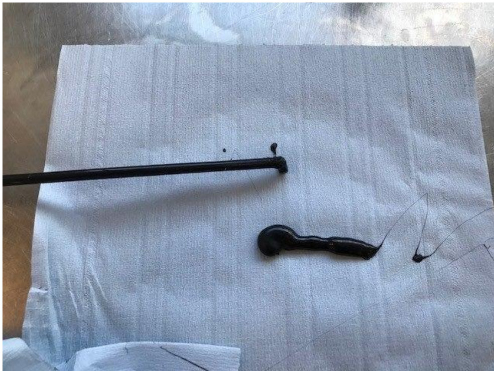
Figure 22: Clearing the component adhesive sealant after prolonged storage.
