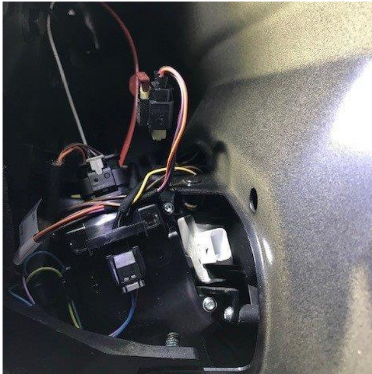
Figure 20: The connector is unplugged from the charging indicator.
