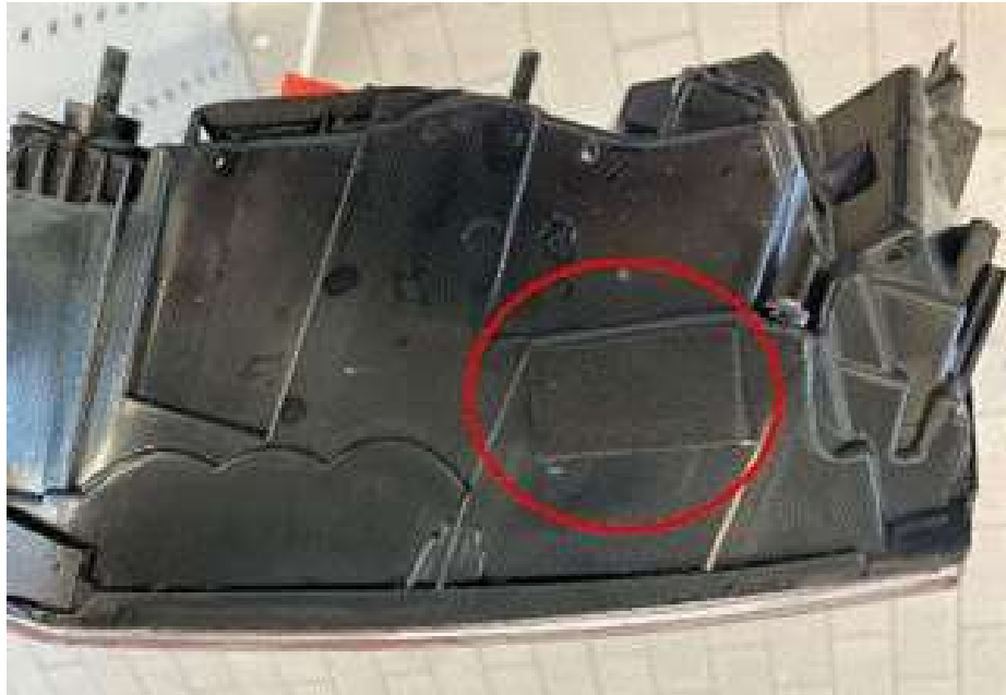
Figure 3. Remove the buffer foam from the taillight.
