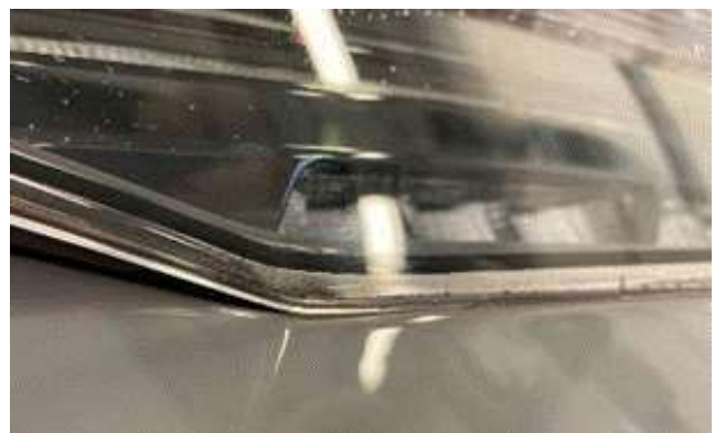
Figure 1. Taillight chafing against the paintwork on the rear lid.
