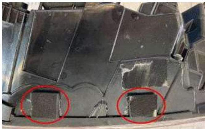
Figure 4. Buffer foam in their new position.
