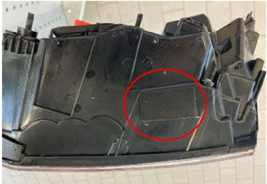
Figure 3. Remove the buffer foam from the taillight.
