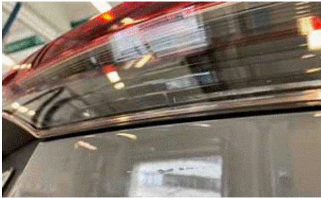
Figure 5. Gap between the taillight and the rear lid.
