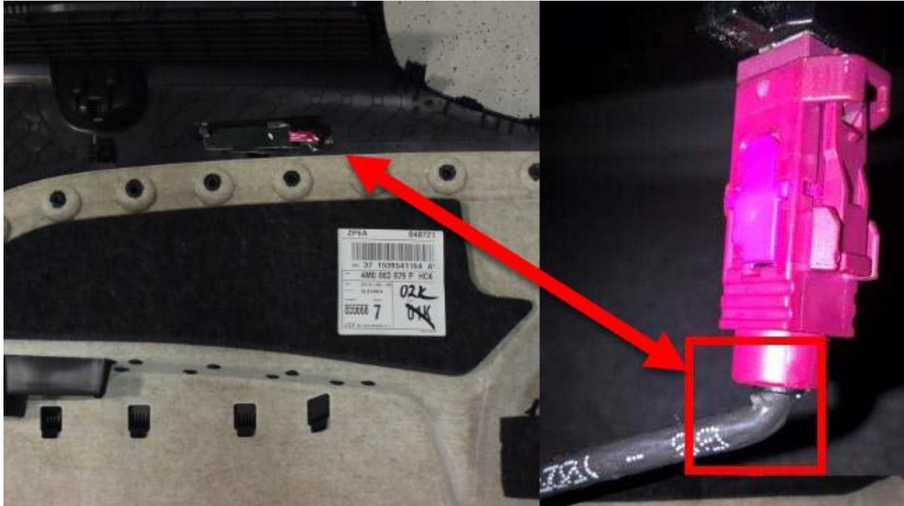
Figure 2. Coaxial wire kinked at R263 SOS Antenna.
