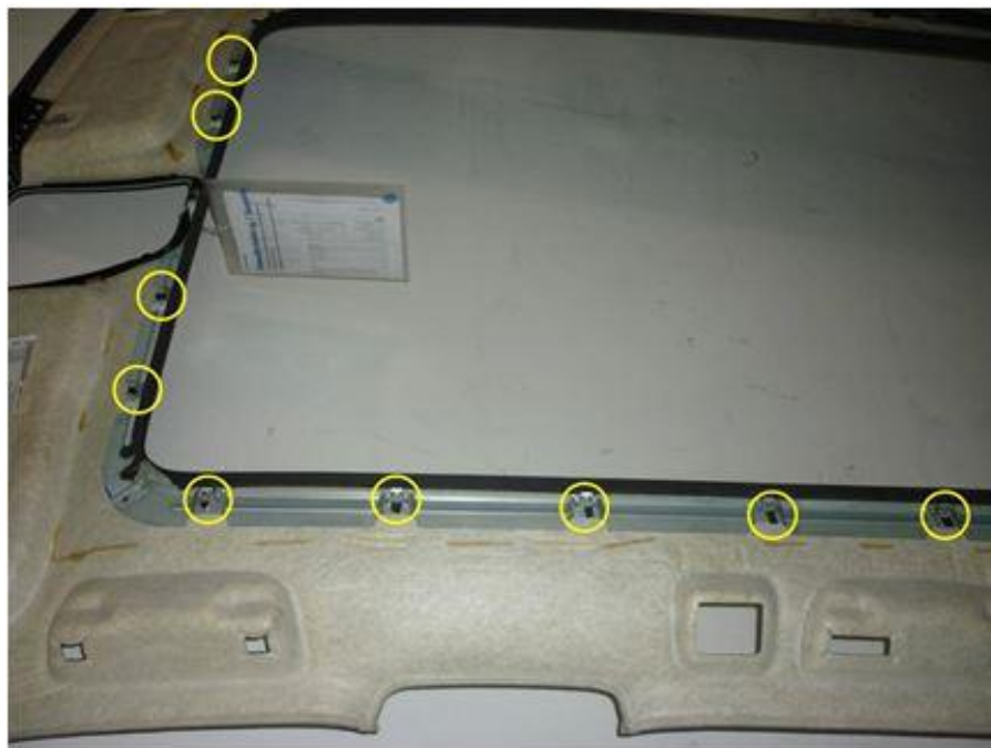
Figure 1. Felt on headliner fasteners.
