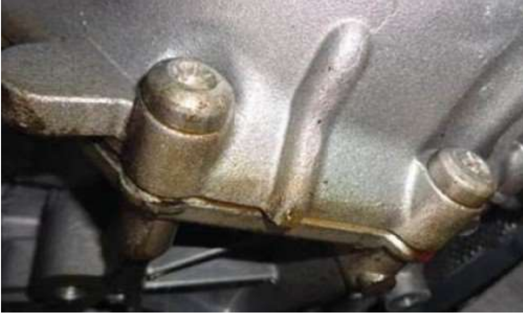
Figure 3. Leak between intermediate housing and end cover
