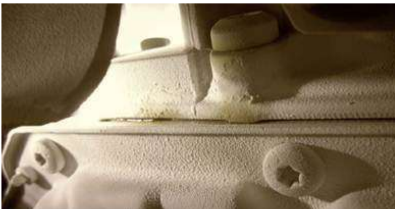
Figure 1. Leak located with talcum spray.
