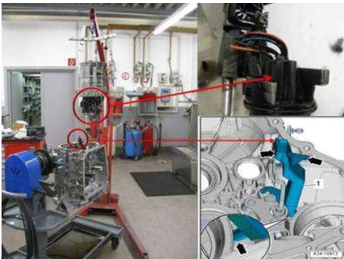
Figure 2. Caution points: drip tray Sensor module connector.
