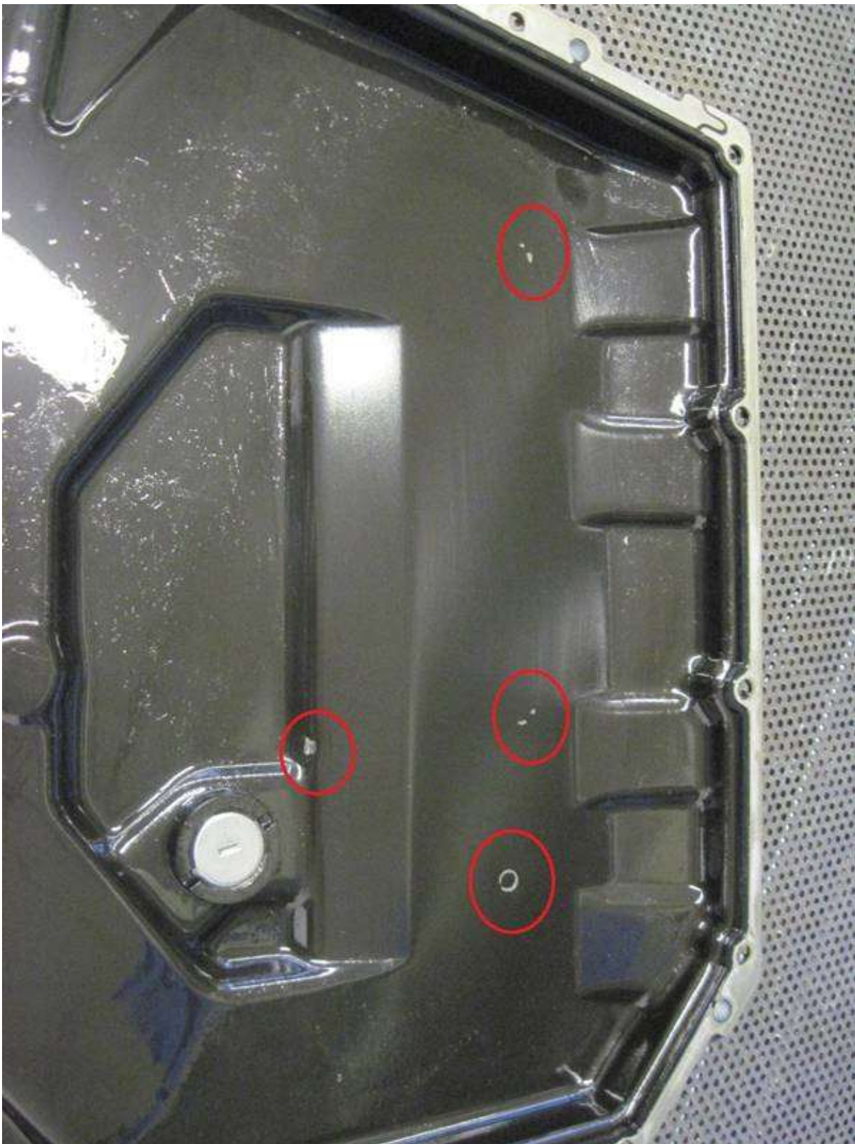
Figure 4. Damaged oil pan because of loose bolts.
