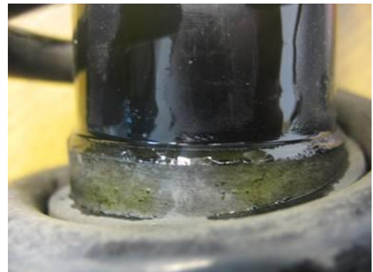
Figure 1. A leaking shock absorber.
