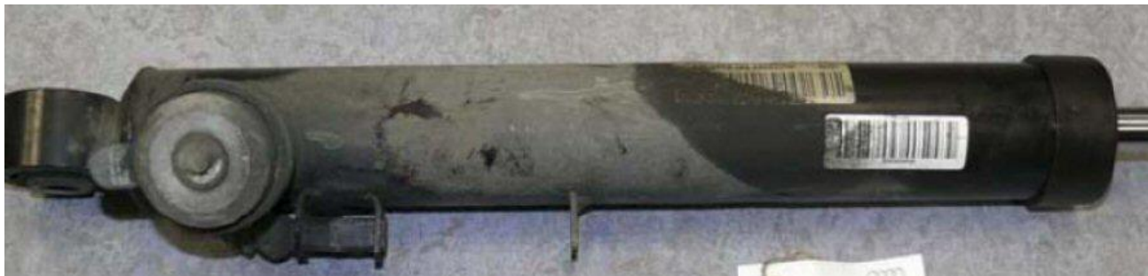
Figure 4. A shock absorber that is not leaking.
