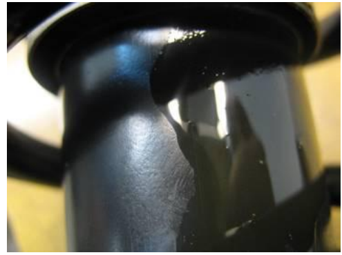
Figure 2. A leaking shock absorber.
