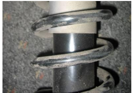
Figure 3. A shock absorber that is not leaking.
