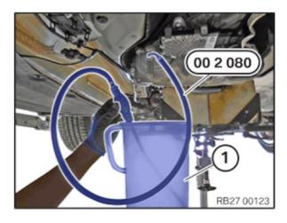
Top up the transmission oil up to the lower edge of the opening for the oil filler plug using special tool 0 493 337 (00 2 080). Use DTF-1 PN 83 22 2 409 710 (@ 0.7 liter).
