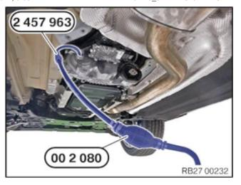
Extract the transmission oil from the transfer case (VTG) using special tool 0 493 337 (00 2 080) and special tool 2 457 963.
