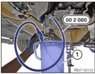
Top up transmission oil up to the lower edge of the opening for the oil filler plug using special tool 0 493 337 (00 2 080). Use DTF-1 P/N 83 22 2 409 710 (@.7 liter)
