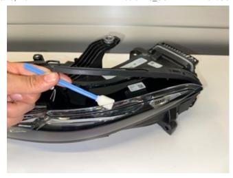
2. Using a cleaning swab, clean the upper channel on the DRL headlight(s).
