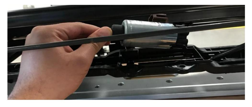
9. Reinstall the inboard side flex cable and cover tube into the motor carrier clips.
