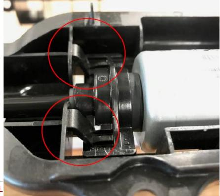
6. Use flathead screwdrivers to carefully disengage one of the motor carrier spring clips. That allows you to pivot the motor upwards without removing the opposite side flex cable.
