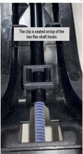
NOTE: If this locking clip has come loose due to the cable popping free, it should be replaced.
