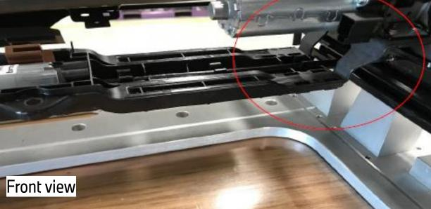
3. Measure the misalignment on both rails and compare how much the difference is. Note: Do the same process for the right side and the left side.
