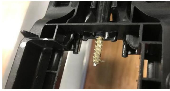
10. Insert the flex cable into the motor and loosely reseat motor into motor carrier tray.
