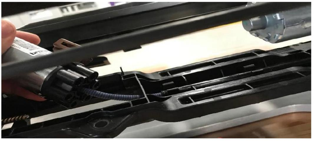
11. Move flex cable in the inboard direction so it is properly seated into the rail gearbox.
