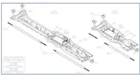
The plastic SLV Motor Carrier tray is available with flex shaft kits.
