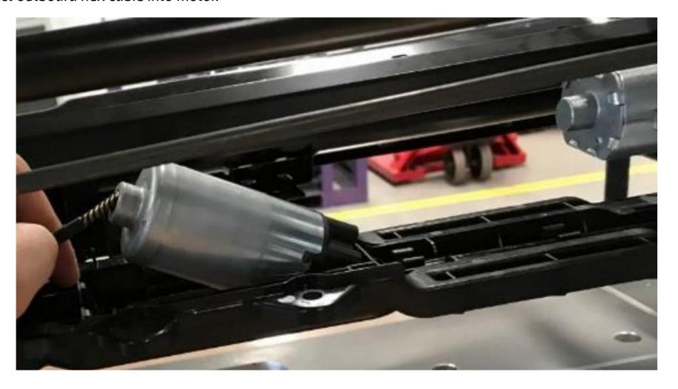
13. Make sure the flex shaft is fully inserted into the electric motor and then push the flex shaft down into the plastic clips holding it in place.
