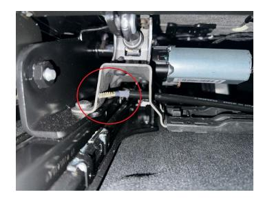
In vehicles equipped with the second row 60% / 40% split seat, the flex cable assembly can come out of the seat rail mechanism (circled). This stops the forwards and backwards travel of the seat.
