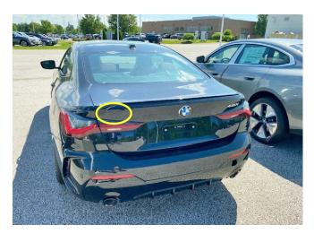
On G22 and G23 xDrive vehicles, the "xDrive" emblem was not installed on the left side of the trunk (circled). Only the "430i" emblem was installed to the right side of the trunk.
