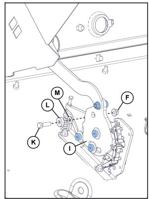
**16.** Install one new screw **(3)**, one new nut **(2)**, retained bearing **(L)**, and washer **(M)** in control bar assembly **(I)**. Torque screw to 20 ft-lb (27 Nm).
