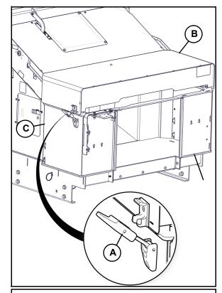
**3.** Open rear shield **(B)** using spring cylinder **(D)** for support.
