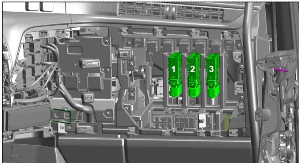
View of the Cab Electrical Center with the Cab FRC Removed 1: IP PDC 2: BB(a) PDC 3: BB(b) PDC
