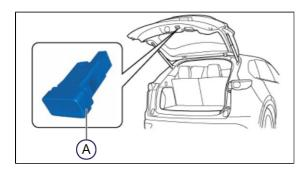
Some Mazda3, CX-30 and MX-30 customers may complain that the vehicle door locking system does not work when the door lock switch on the liftgate interior trim is pressed. DTC B11C4:23 (BCM - liftgate lock switch circuit malfunction) may be stored. This may be caused during a high pressure car wash and/or condensation. Water may enter through the rear center brand emblem base component and drip onto the switch connector causing corrosion. The rusted connector may also cause a battery drain.
