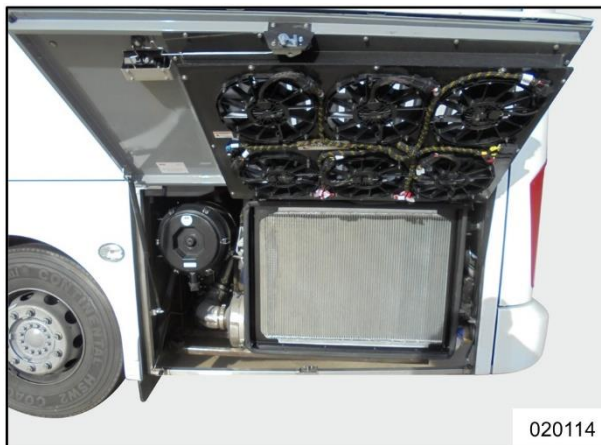
Figure 1: Radiator compartment on CX45
