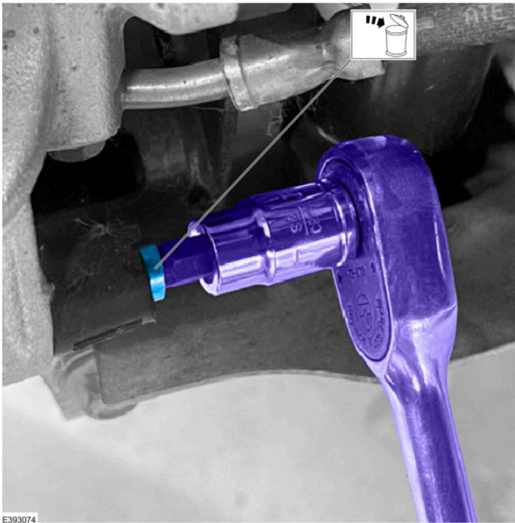
6. Loosen the upper guide pin and rotate the rear caliper upwards to access to the bushing housing. (Figure 6, Callout 1)
