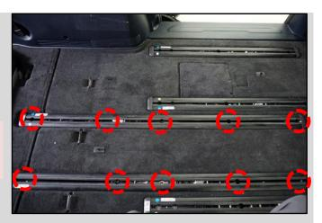
Loosen the two (2) end cap cover (I) retaining screws for the <u>RIGHT</u> 2<sup>nd</sup> row <u>inner</u> and <u>outer</u> seat rails.
