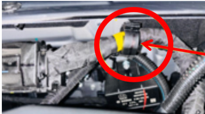
Fig. 4 Harness Routing Clamp
