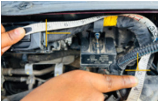
Fig. 1 PCM Harness Measurement
