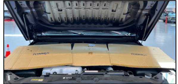
Figure 1. Example of Engine Covered with Equivalent Protective Material
