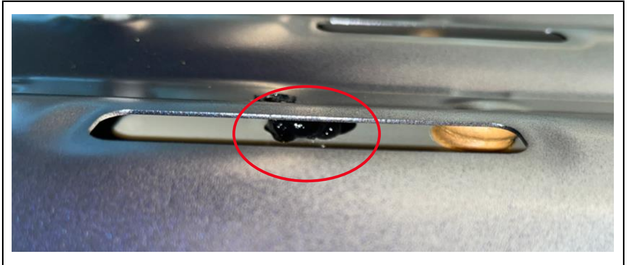
Figure 8. 3M™ NVM Dampening Material Approximately 25 mm
