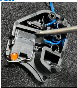
The dimensions on the original factory-installed right side second-row seatback rest microswitch assembly may not be correct. If so, this causes the microswitch to move when the seat backrest is raised to the upright seating position.
