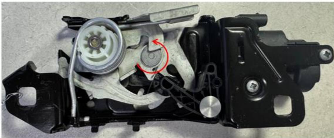
Fig 1. Latch In Closed State With Hood Open. Red Arrow Shows Direction Latch Needs To Rotate To Unlatch.
