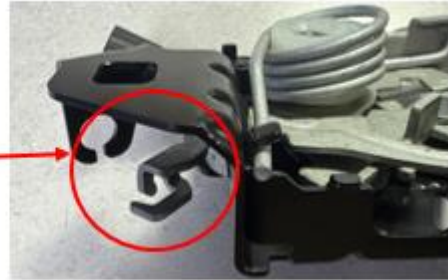
Fig 2 Manual Release The Latch By Actuating 2 times.
