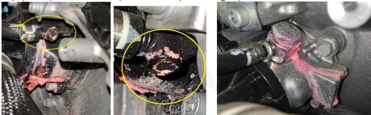
Sample pics. of Crossover – Engine Coolant leak
