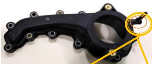
1) Sample pic. of Crossover built in Plastic Material (more frequent coolant leak area highlighted).
