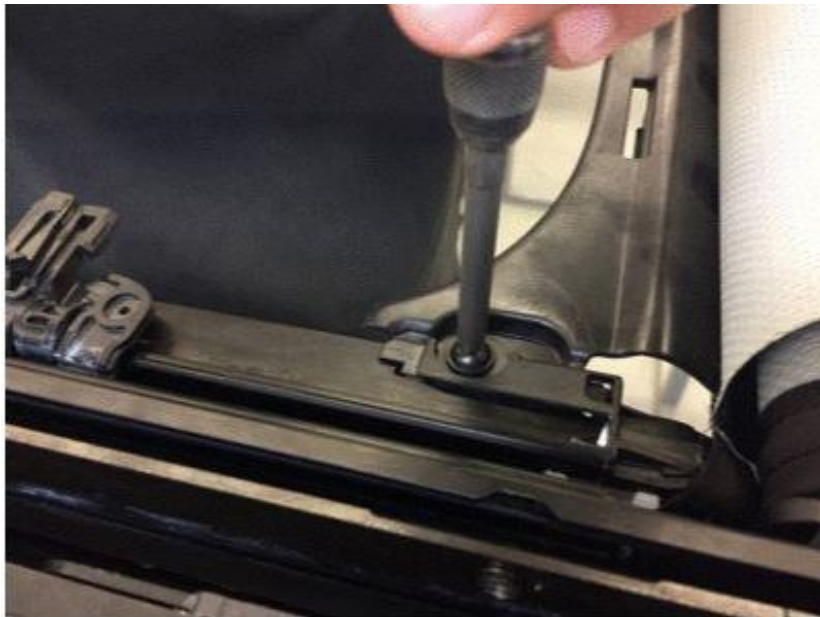
Figure 12. Tighten bolt to 3 Nm.
