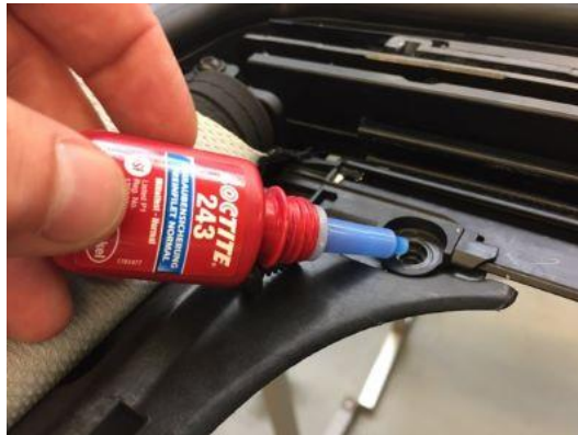
Figure 11. Locking compound application.
