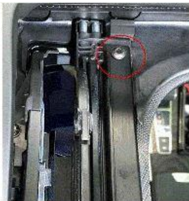
Figure 13. Loosen the bolt a few turns but do not unscrew completely.
