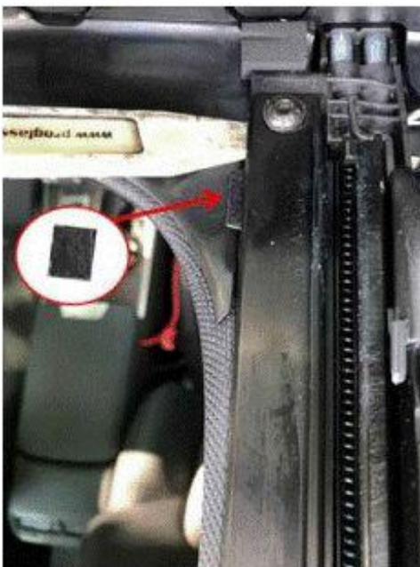
Figure 13. Loosen the bolt a few turns but do not unscrew completely.
