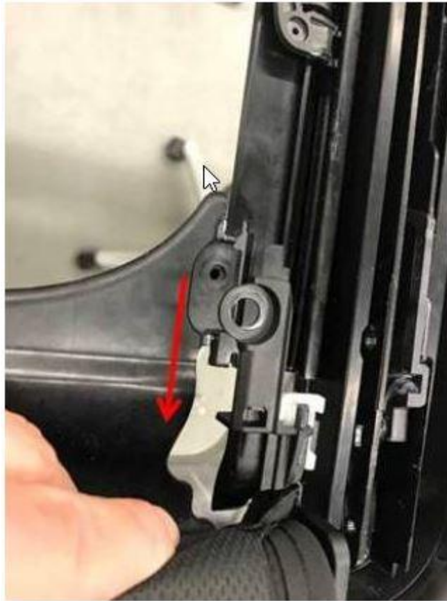
Figure 6. Roller blind moved toward rear.
