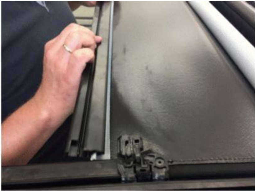
Figure 3. Move the blind back.
