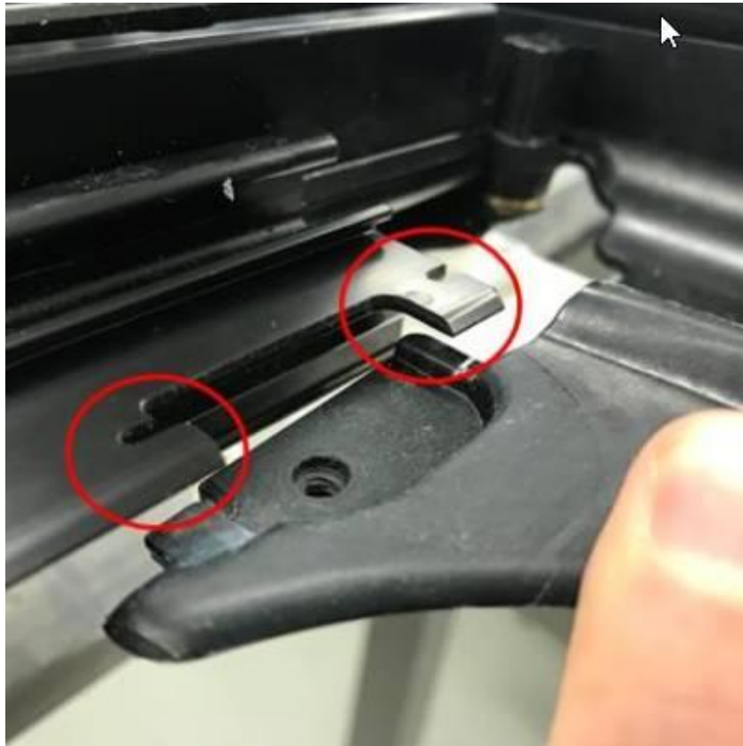
Figure 7. Areas to clean using cleaning solution D 009 401 04.
