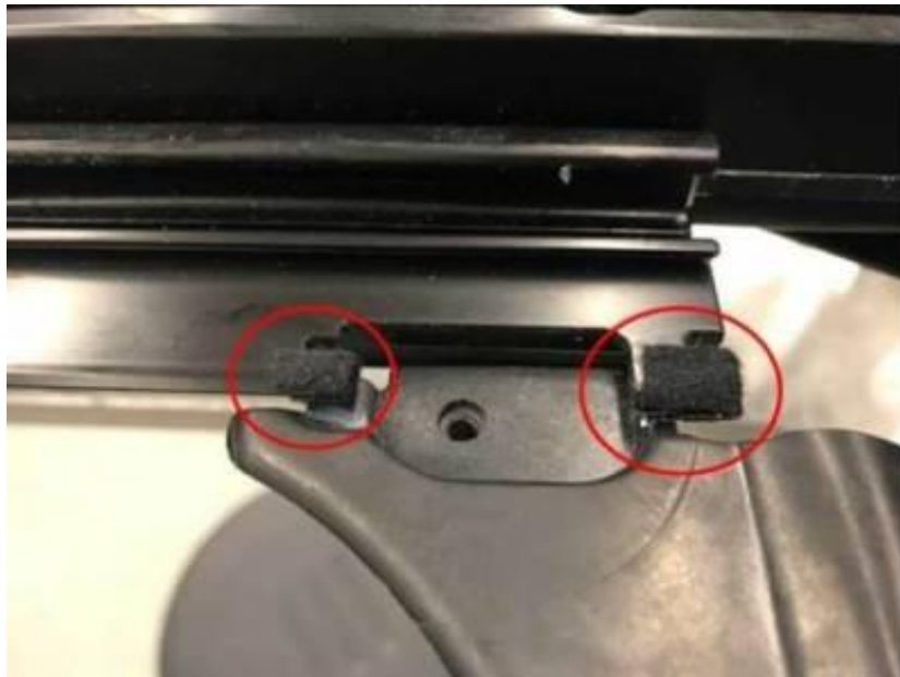
Figure 9. Felt pieces bonded.
