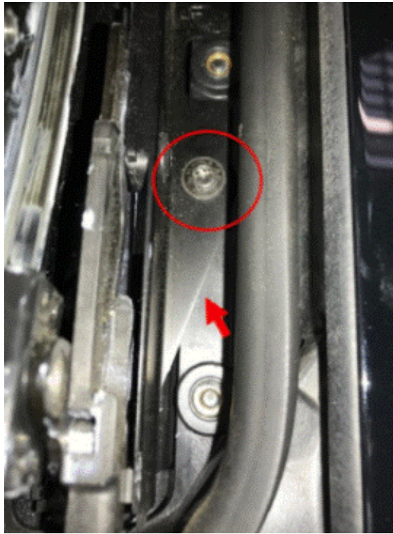
Figure 17. Loosen the bolt a few turns, but do not remove.
