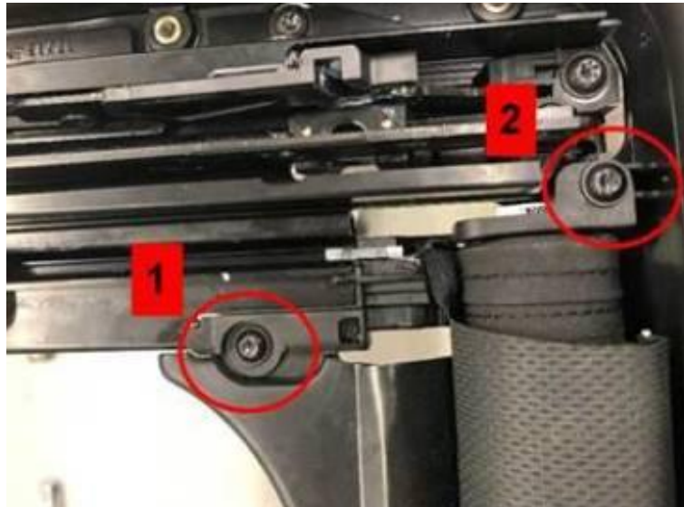
Figure 5. Remove the bolts.
