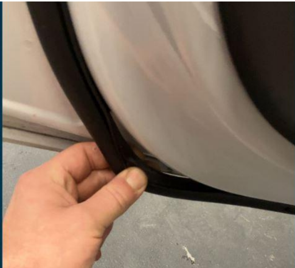
Figure 1. Door seal coming loose.
