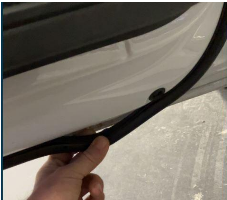
Figure 2. Door seal coming loose.
