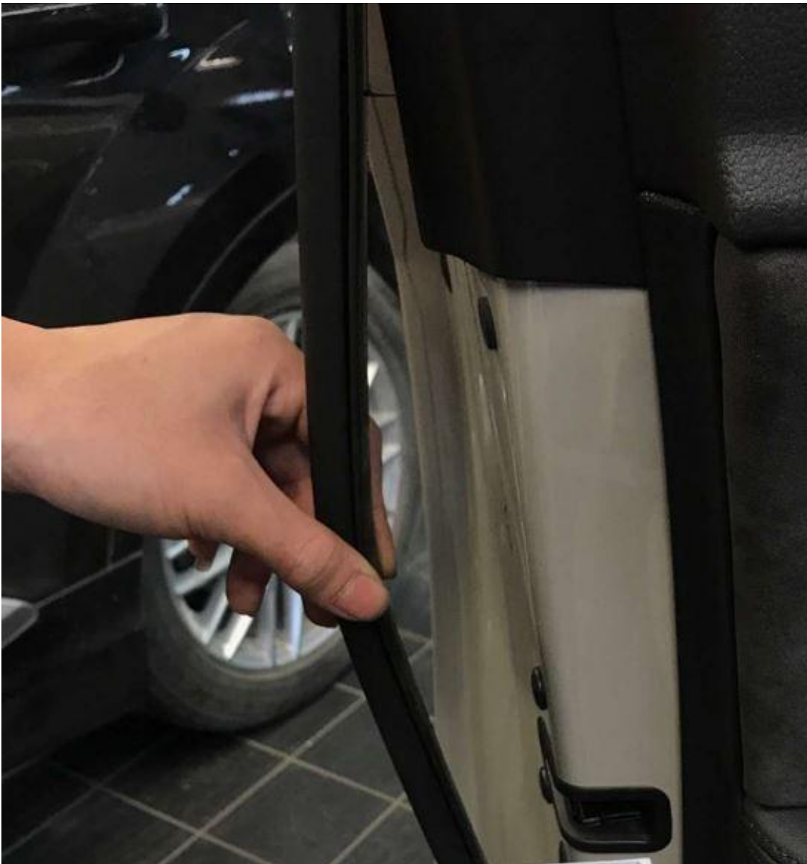
Figure 4. Door seal coming loose.
